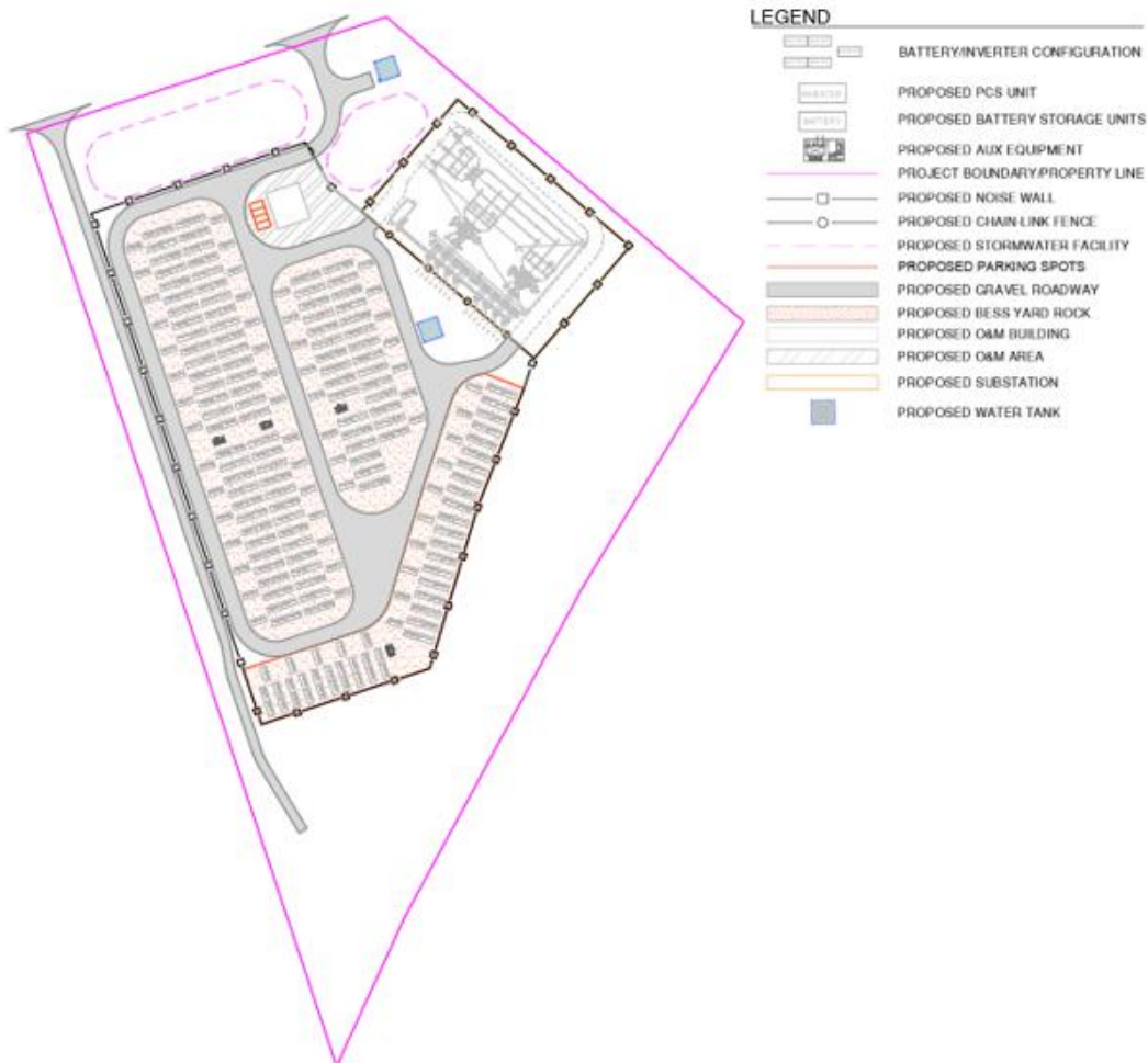
Figure 2 General Equipment Arrangement
